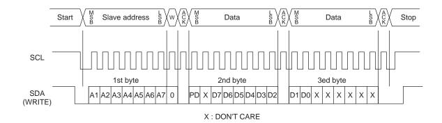
The standard data transfer to this device consists of three bytes: the slave address of the first byte and the data of the second and third bytes.
